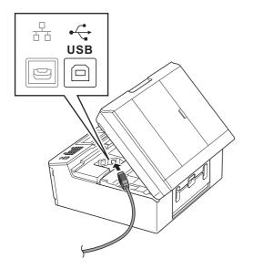
Carefully guide the USB cable into the cable channel and out the back of the machine. Connect the cable to your computer.
